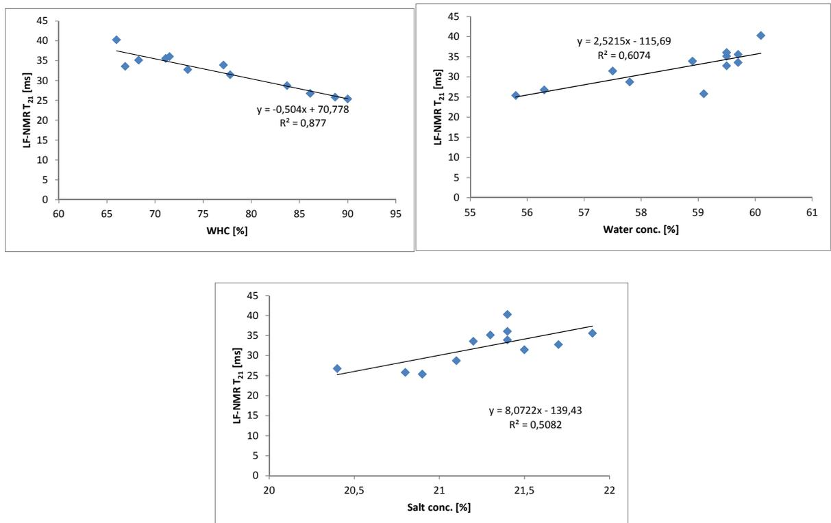
Figure 3: Partial Least Square Regression models of LF-NMR  $T_{21}$  relaxation time to WHC, water and salt content respectively.
