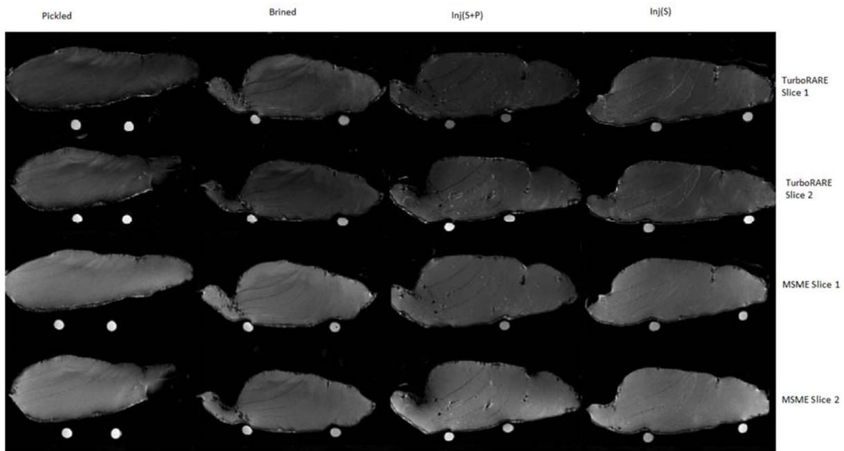
Figure 4:  $^1\text{H}$  MRI cross-sectional images of dry salted cod fillets using TurboRARE (above) and MSME (below) pulse sequences. Light circles indicate reference salt solutions. Two slices from each treatment are shown.
