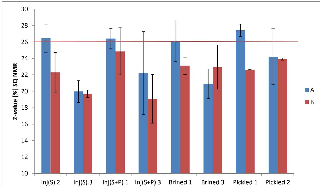
Figure 11: Z-salt value based on SQ  $^{23}\text{Na}$  NMR analysis. Red horizontal line indicates fully saturated salt brine (26 %).
