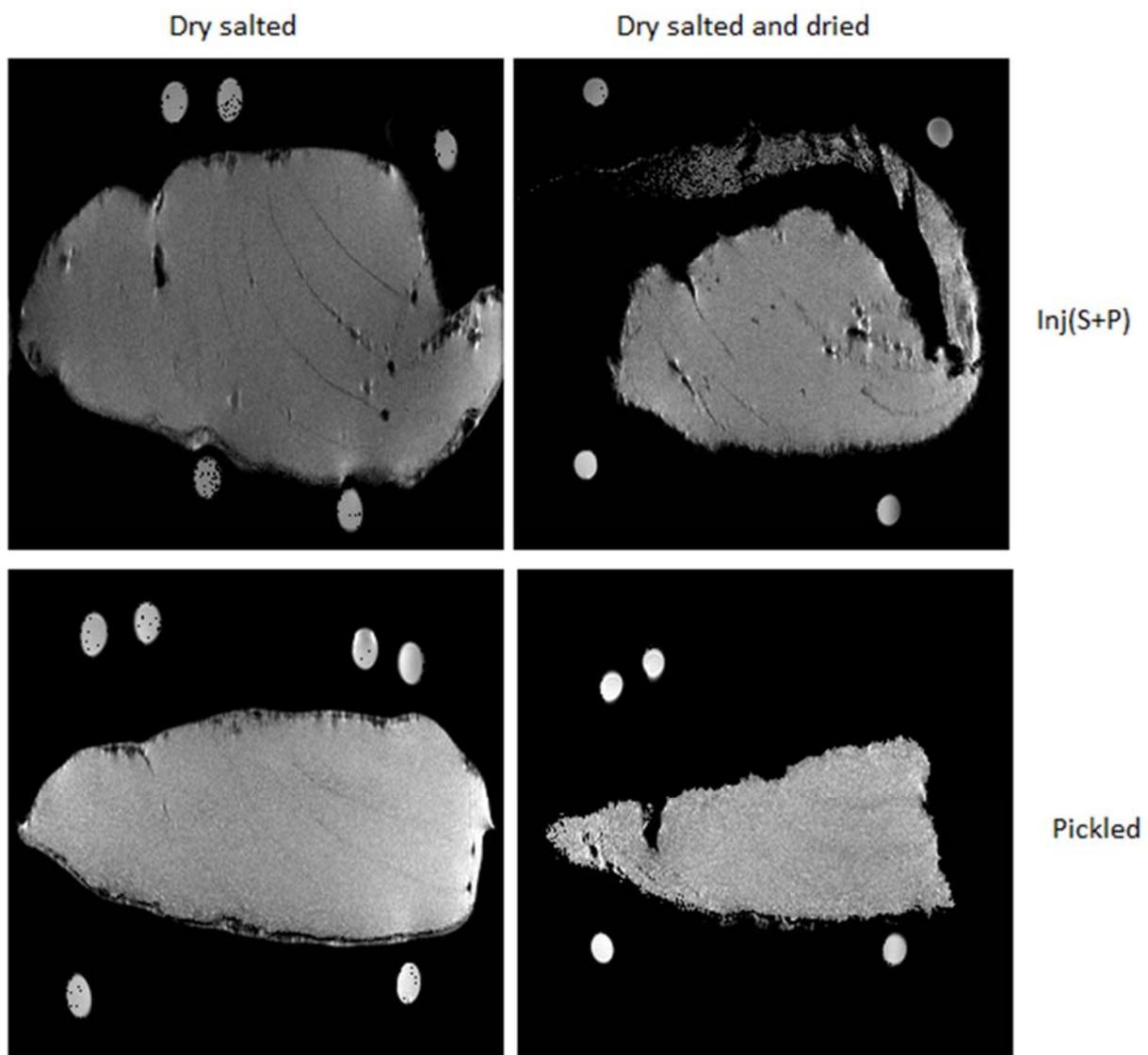
Figure 14:  $^1\text{H}$  MRI cross-sectional images of dry salted cod fillets using the MSME pulse sequence. Light circles indicate reference salt solutions.
