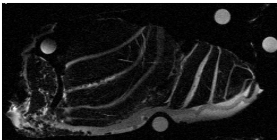
Figure 7: TurboRARE image of brine injected (Inj(S)) fillet after 24 h in the magnet. Light circles indicate reference salt solutions.
