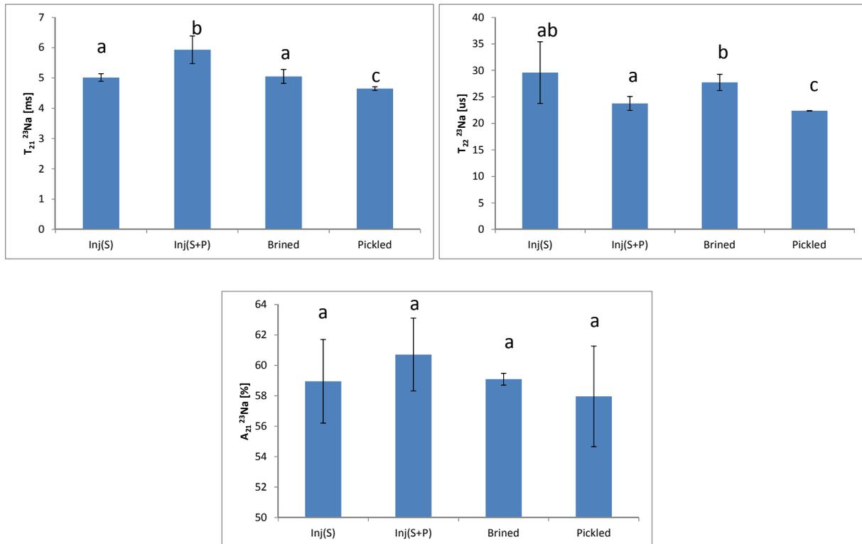
Figure 11: Sodium relaxation times for dry salted cod of different pre-salting methods.
