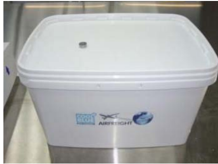
Figure 8. Ibutton temperature logger on top of a Cool Blue Box.
