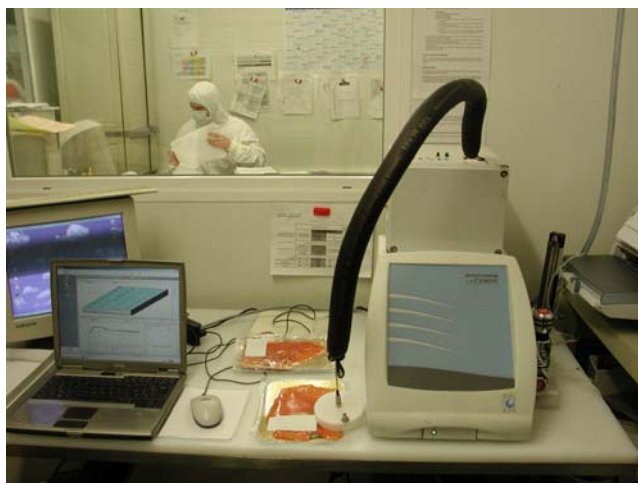
Figure 2: On site testing at one of the smokehouses showing the FishNose with the sampling system developed in the project.
