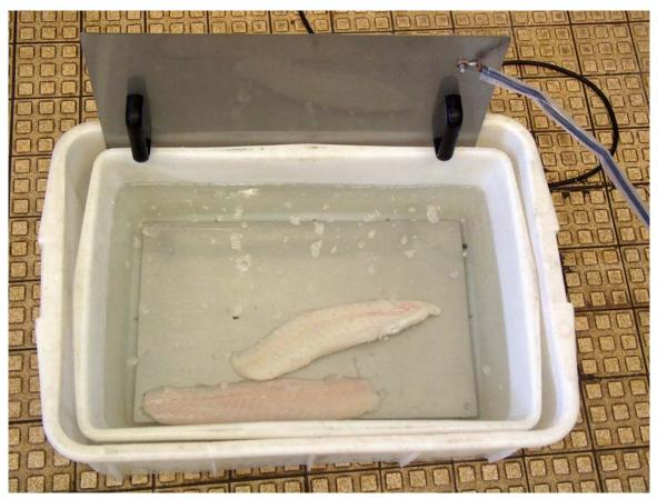
Figure 3. Samples of cod in container between two parallel stainless electrodes
