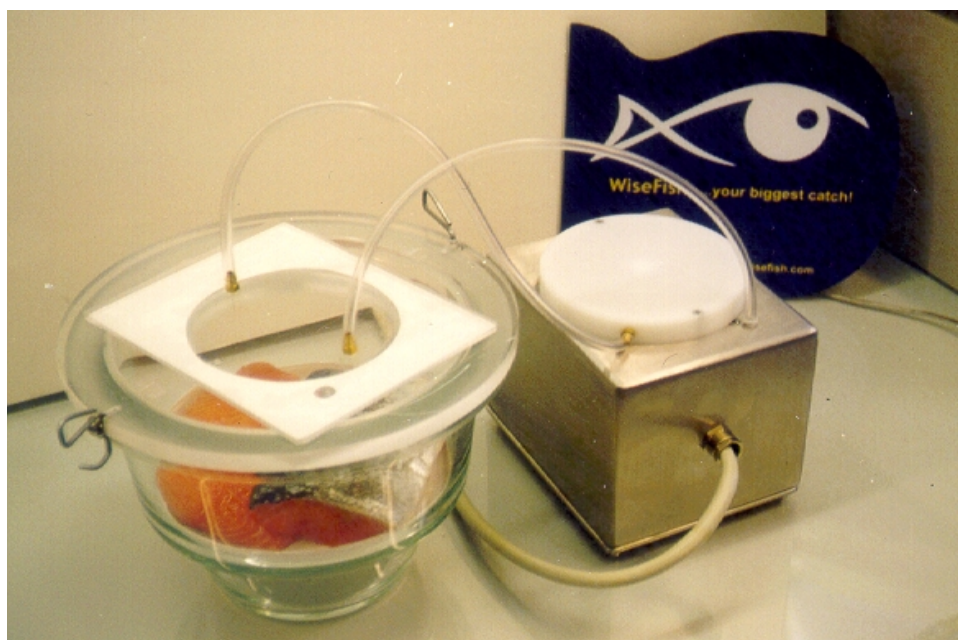
Figure 4. The new version of the electronic nose FresSense with the electrochemical gas sensors (CO, H 2 S, SO 2 , NH 3 ) developed by Bodvaki and Icelandic Fisheries Laboratories. A pump ensures the transport of headspace from the closed glass sampling container (a) to the measurement chamber (b).
