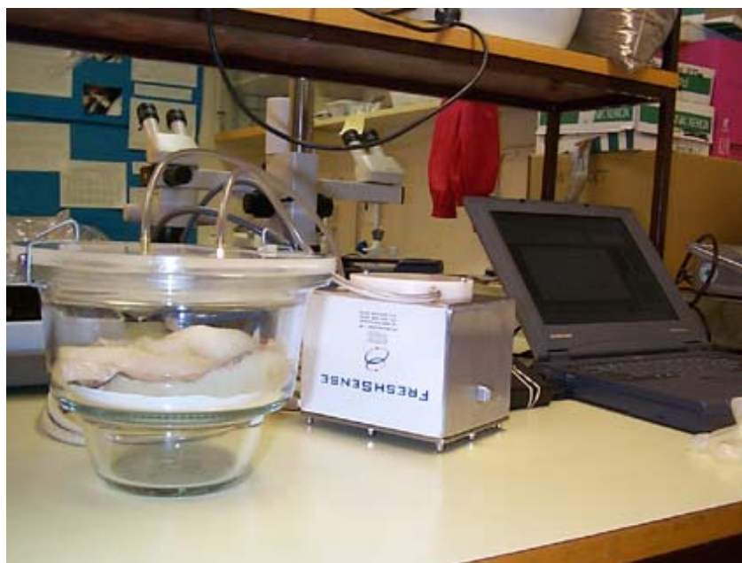
Figure 2. The electronic nose FreshSense with the electrochemical gas sensors (CO, H 2 S, SO 2 , NH 3 ) developed by Bodvaki and Icelandic Fisheries Laboratories.
