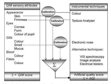
Fig. 1. Construction of the Artificial Quality Index (AQI). After calibration with sensory data (Quality Index Method (QIM)) the instrumental readings are combined into Artificial quality score giving the AQI (adapted from Di Natale, 2003).
