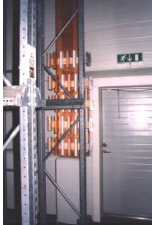
Figure 1. Gluelam samples in salt fish storage
