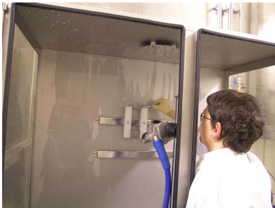
Figure 2. The semi-automated washing station enabled a controlled washing protocol to be executed. Detergent concentration, temperature, water pressure and distance from sample plate was all standardised and monitored between experiments.
