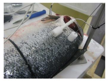
Figure 4 Testor logger sensors placed in a salmon
