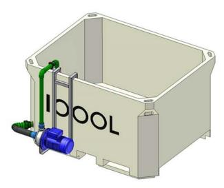
Figure 1 Schematic figure of the sub-chilling tub equipped with a centrifugal pump to recycle the chilled brine.
