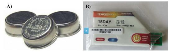
Figure 3. A) IButton DS1922L temperature loggers used to monitor the temperature within the product and the ambient temperature. B) Tempsen ITAG-PDF single use temperature logger used to monitor the temperature of product and the ambient temperature.
