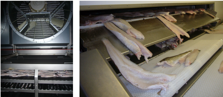
Figure 2.1: Precooling of whitefish fillets in a SuperChiller (Valtýsdóttir, 2011b). Fillets are subjected to both blast and contact cooling as they are transferred with the skin down on an aluminium belt while cold air is blown above them (left). Superchilled fillets exit the SuperChiller (right) before being transferred on another conveyor belt to deskinning and trimming.
