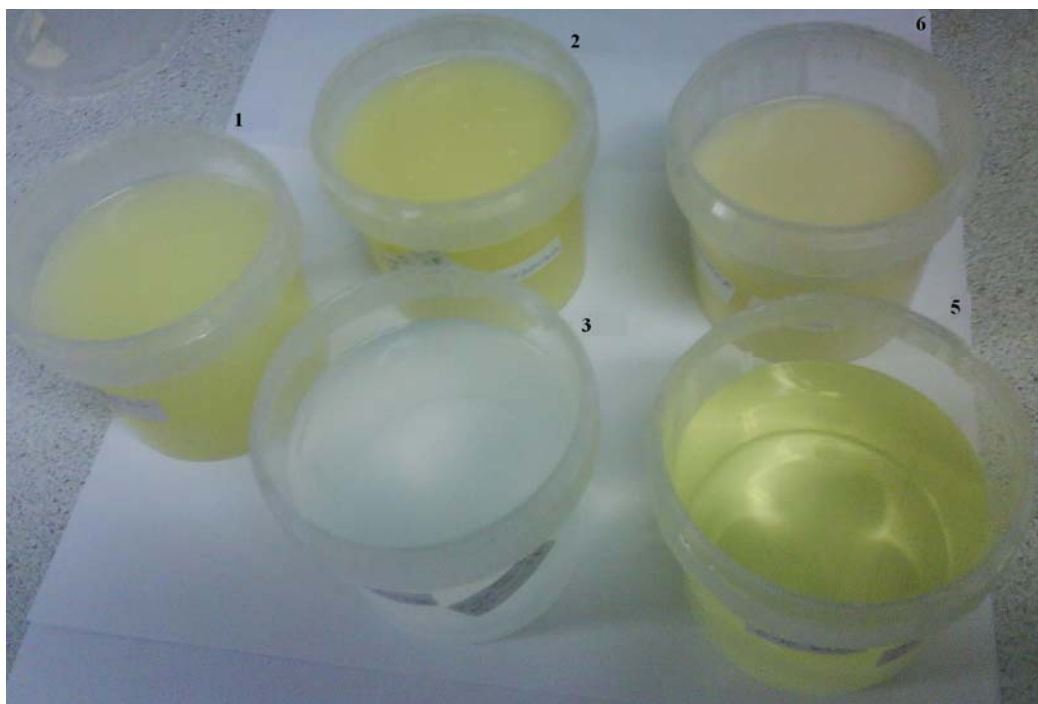
Fig. 3 Crude whey and filtrated whey. Crude 1, nano-filtrated concentrate 2, nano-filtrated permeate 3, ultra-filtrated concentrate 4, ultra-filtrated permeate 5.
