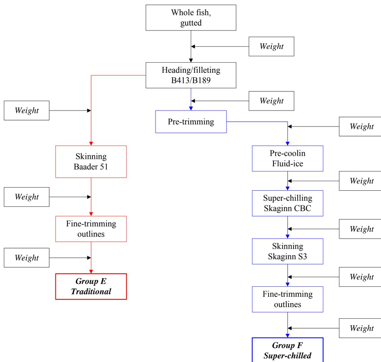
Figure 2 Main (II) experiment layout
