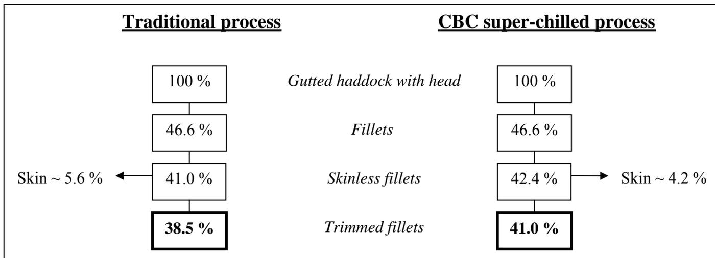
**Figure 17** The process yield from whole gutted haddock with head.
