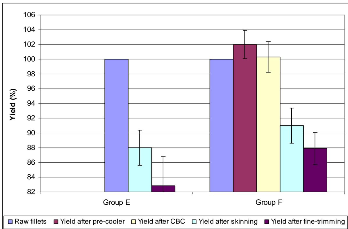
**Figure 16 Yield after the processing steps. Group E = Traditional process. Group F = CBC super-chilling process.**
