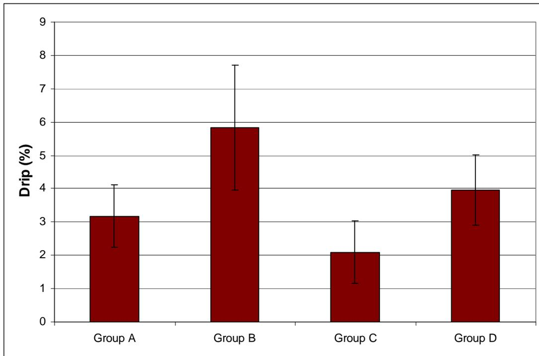
**Figure 6** Drip after 6 days storage at  $-1.0^{\circ}\text{C}$ . Group A=Traditional + skinless. Group B=Pre-cooler + skinless. Group C=Pre-cooler + CBC + skin on. Group D=Pre-cooler + CBC + skinless.
