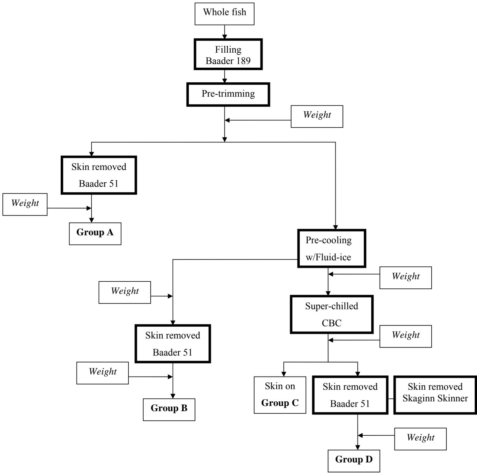
Figure 1 Preliminary (I) experiment layout.
