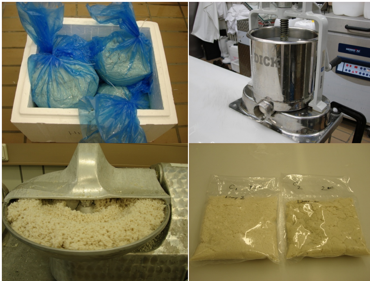
2.5 Receiving, dewatering, mixing with cryoprotectants and packing of haddock protein isolates
