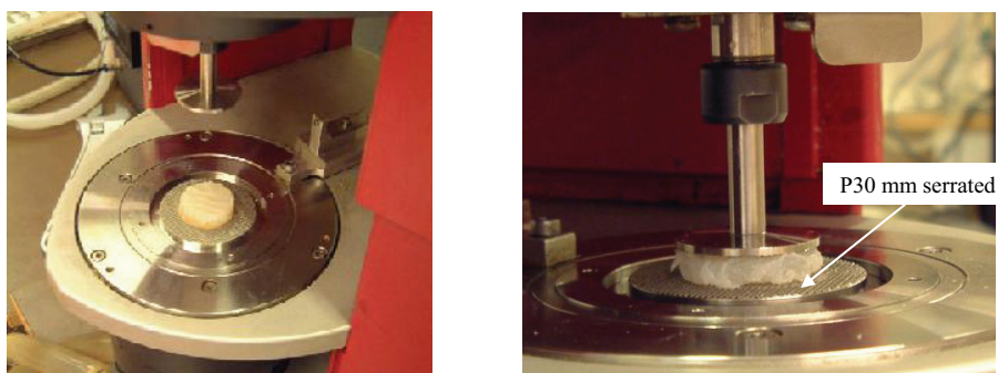
Figure 39. Measurements on salted fish samples in a StressTech rheometer
